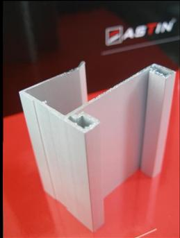
**ORIENT** - aluminium profile is used with 16-18 mm. thickness door fillers (except glass products), has adhesive amortization brush, with only one matt anodized shade (silver). Recommended door height is up to 2700mm., width up to 900mm. The front edge of the profile can be assessed by 1mm. thickness wood imitation PVC or HPL, which provides a unique charm to sliding door and is easy adaptable to the room interior.
