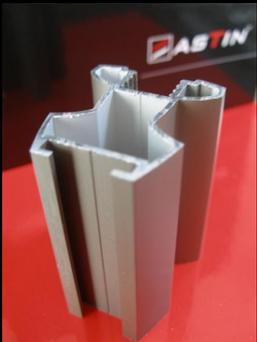
**TWINS** - modern and unique aluminium profile with stud aluminium tape and amortization brush, which covers all of the holes made during door manufacturing proces. Used with 4-10 mm. thickness door fillers (chipboard, glass products, rattan, etc.). There are 4 matt anodized shades (silver, gold, light brown and dark brown). Recommended door height is up to 2700mm. (if with supplementary agreement, door can be made up to 3500 mm. height), width up to 1500mm.
