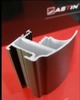
**NEW HEROS** – aluminium profile with stud aluminium tape and amortization brush, which covers all of the holes made during door manufacturing proces. Used with 4-10 mm. thickness door fillers (chipboard, glass products, rattan, etc.). There are 4 matt anodized shades (silver, gold, light brown and dark brown). Recommended door height is up to 2700mm. (if with supplementary agreement, door can be made up to 3500 mm. height), width up to 1500mm.
