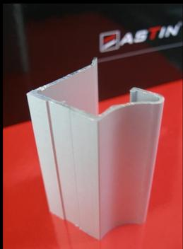
**FIONA** – minimalist and narrow aluminum profile is used with 16-18 mm. thickness door fillers (except glass products), has adhesive amortization brush, with only one matt anodized shade (silver). Recommended door height is up to 2700mm., width up to 900mm.
